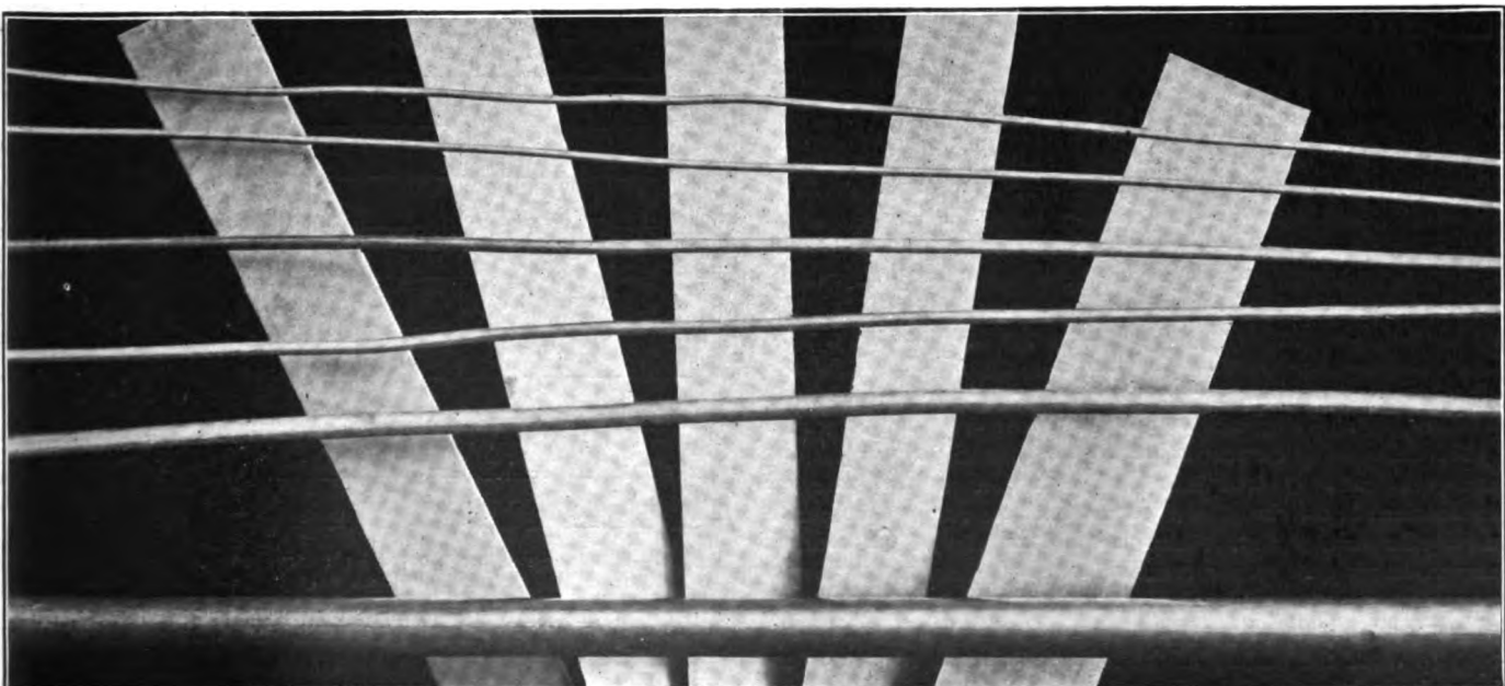
Fig. 3—Depicting several sizes of rolled bars of Duralumin and some of the regularly made strip products
